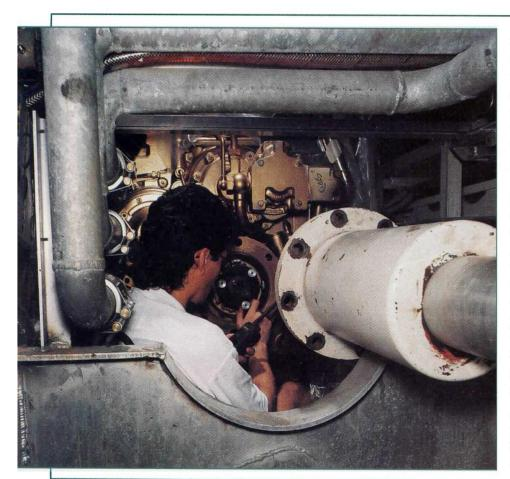
drawbacks. First, old-fashioned artistry calls for a *lot* of intuition and experience. Second, long prop shafts are not really straight enough to produce truly accurate realignments; they droop in unsupported areas, like between shaft logs and reverse-gear output flanges.
