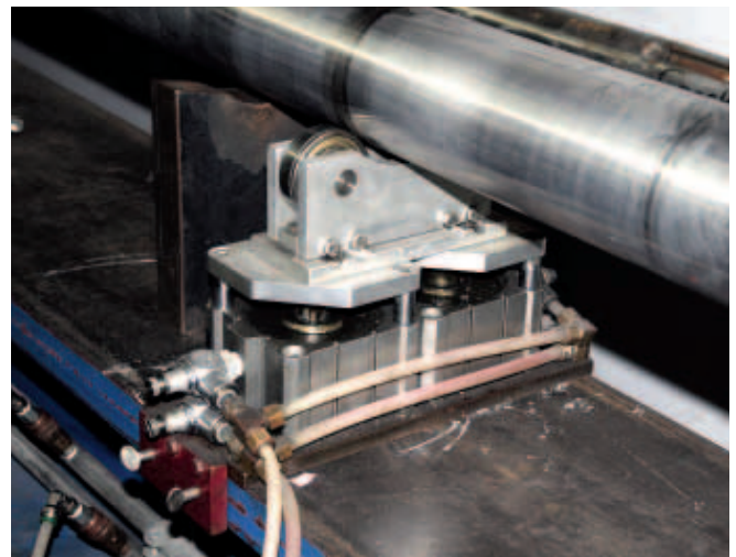
Top: Machinist Chris Zylka prepares to check the run-out on a shaft coupling extension. Above: A pneumatic jack used to support shafts as they are measured and straightened.
