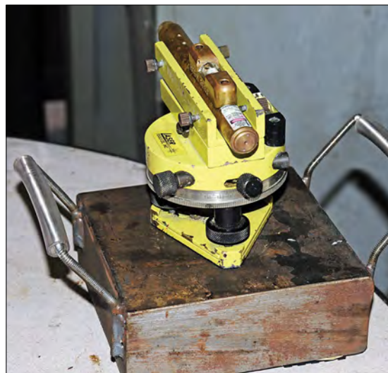
Left —Chris Brown checks alignment with an optical scope, a precise method involving three glass targets. Right —While High Seas primarily measures alignment with optical scopes, it also employs lasers for a process called deck spotting, which measures changes in vessel shape before and after hauling. This laser is attached to a heavy steel plate for stability.
