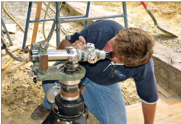
Left —Chris Brown checks alignment with an optical scope, a precise method involving three glass targets. Right —While High Seas primarily measures alignment with optical scopes, it also employs lasers for a process called deck spotting, which measures changes in vessel shape before and after hauling. This laser is attached to a heavy steel plate for stability.
