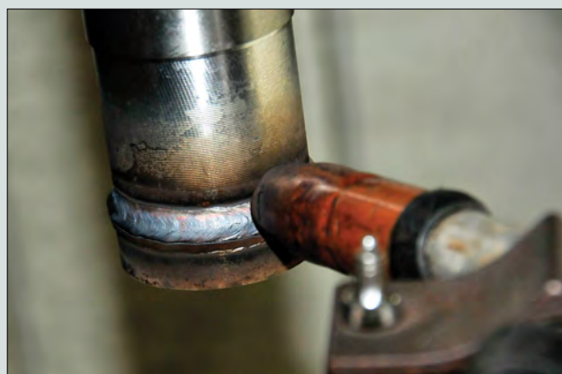
Cladding, or weld-over, can save some defective shafts. Here, a bead of weld metal has been built up over a previously pitted shaft. After it cools and has been turned down in a lathe to match the shaft diameter, the repair will be imperceptible.
