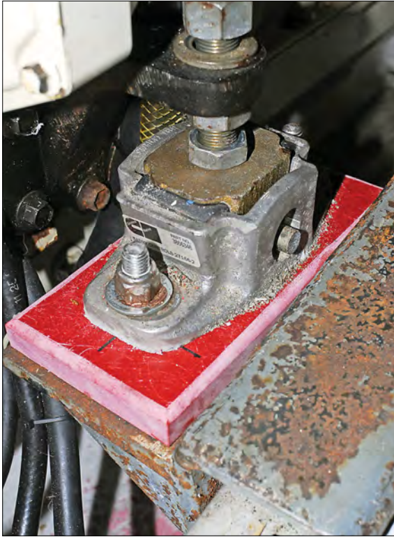
Left —An adjustable motor mount is shimmed to reduce stud extension. Boatbuilders should ensure that an initial engine installation is properly aligned without relying on excessive extension of motor mount studs, which can lead to stud failure. Instead, motor mounts should be thought of as tools for fine-tuning alignment. Above —Alignment between the engine and shaft couplings requires precise measurement, using geometry and feeler gauges, like those shown here. Ultimately, coupling faces must be made parallel and centered with each other to within a few thousandths of an inch.
