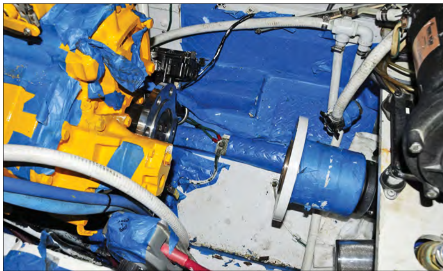
Facing page —Altering the shaft alignment typically requires adjusting the location of the struts. This is often accomplished by making customized shims from thickened epoxy. Here, temporary wedges position a strut while the epoxy shim cures. Left —In most cases, the term alignment refers to the interface between the engine and the shaft couplings, shown here during installation.
